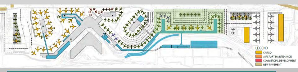
U-shaped concept provides additional aircraft hold positions and operational flexibility
