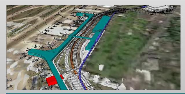
Building 3-D model in AutoCAD to set geometry of facilities in North Terminal area
